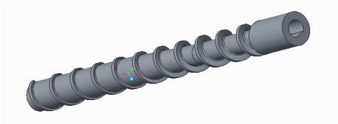
Figure 30. Screw solid model in CREO Parametric.
