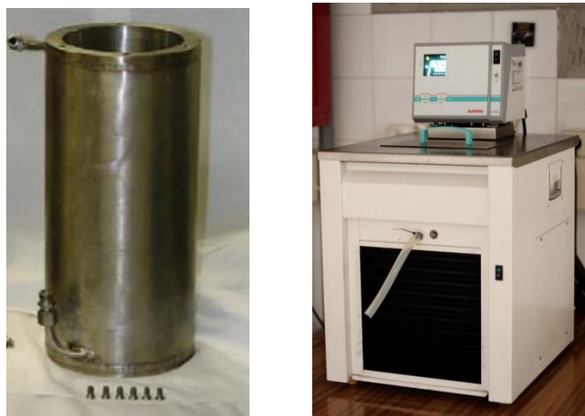
Figure 3.10 Double-walled stainless steel cylinder and refrigerated-heating circulator Julabo FP50-HE.
