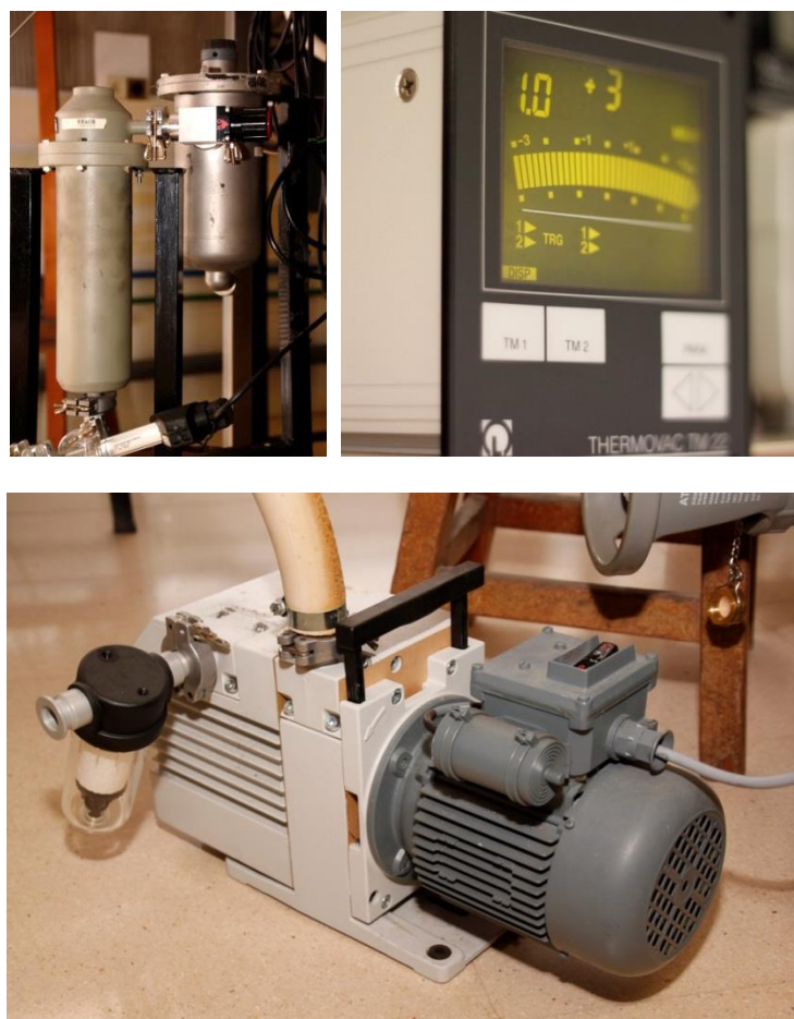
Figure 3.15. Elements of the vacuum system: zeolites trap, cryogenic trap, vacuumeter and vacuum pump.
