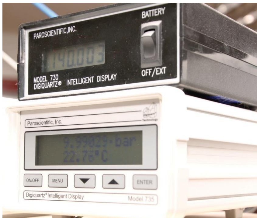
Figure 3.13. Pressure transducers used to measure the pressure in the range (2 - 20) MPa (up) and (0 - 2) MPa (down).
