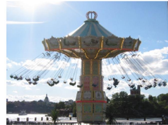
Figure 2. The 48 seat wave swinger rides from Zierer at Gröna Lund, Sweden. The swings are suspended from three circles with slightly different diameters, and slightly different chain lengths. The 16 swings in the outer circle are suspended at a distance of 2 m and the four chains holding the seat are about 5.5 m long, (including the extra chain at the top and the height of the seat).
