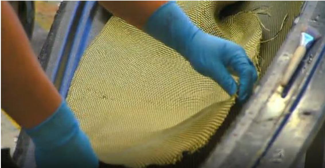
Figure 11.2: Placing the glass fibre into the mould. [21]
