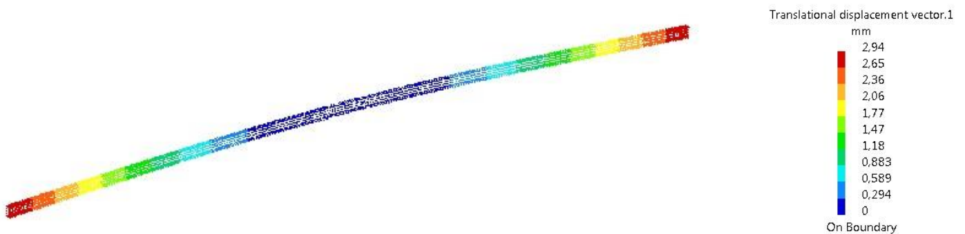
Figure 13.11: Results of the static calculations for the carbon tube case
