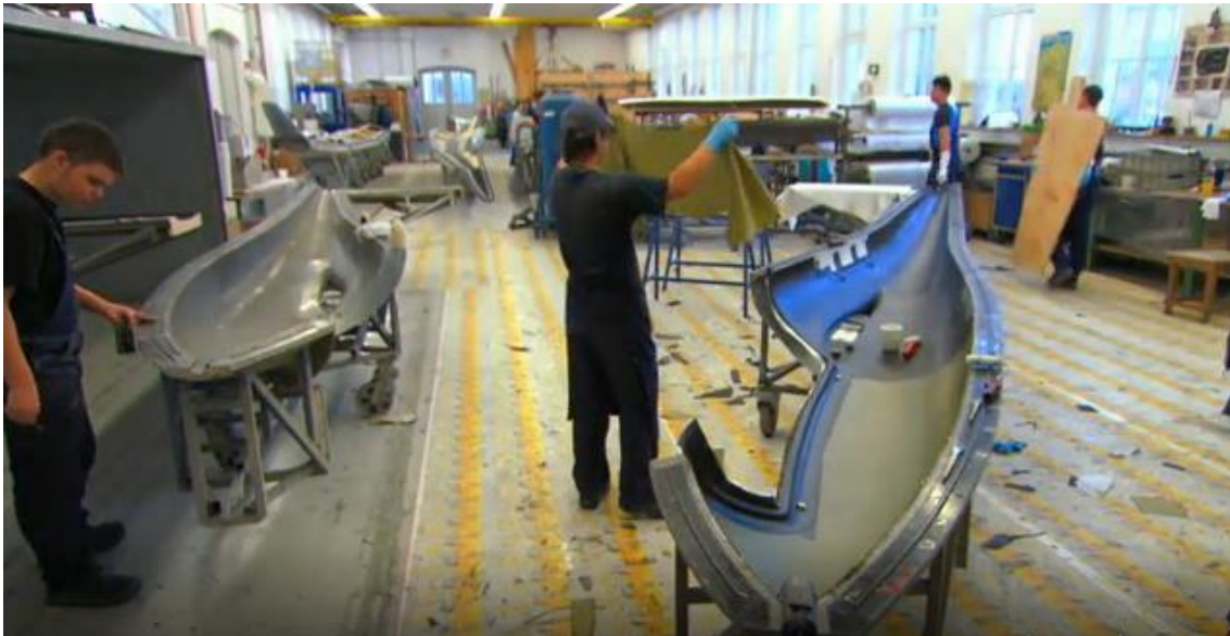
Figure 11.1: Two moulds for the same part of one aircraft, the fuselage. [20]
