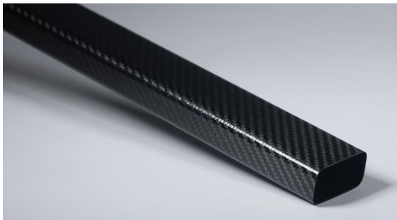
Figure 10.3: Example of a carbon fibre tube similar to the one is used for this UAV.[17]
