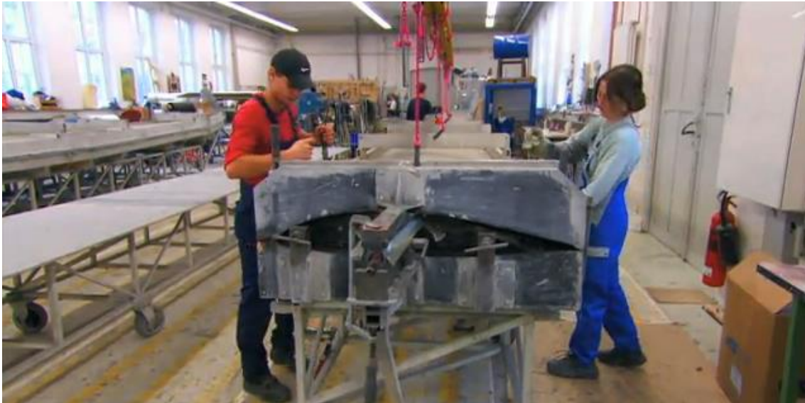
Figure 11.4: Moments before the union of the moulds with pressure and heating. [23]
