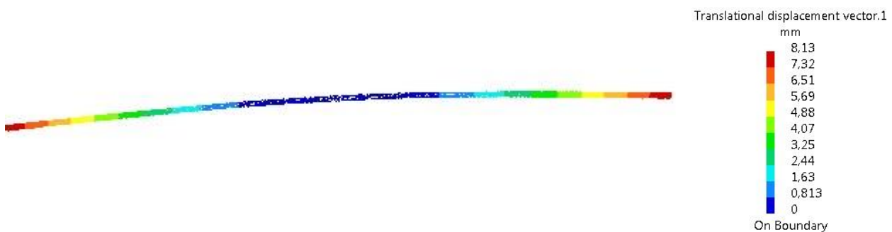
Figure 13.13: Results of the static calculations for the carbon tube case
