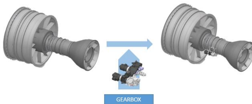
Fig. 8: Brief diagram of the assembly sequence in Station 3.
