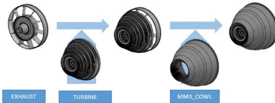
Fig. 4: Brief diagram of the MM3 assembly sequence in Workstation 1.
