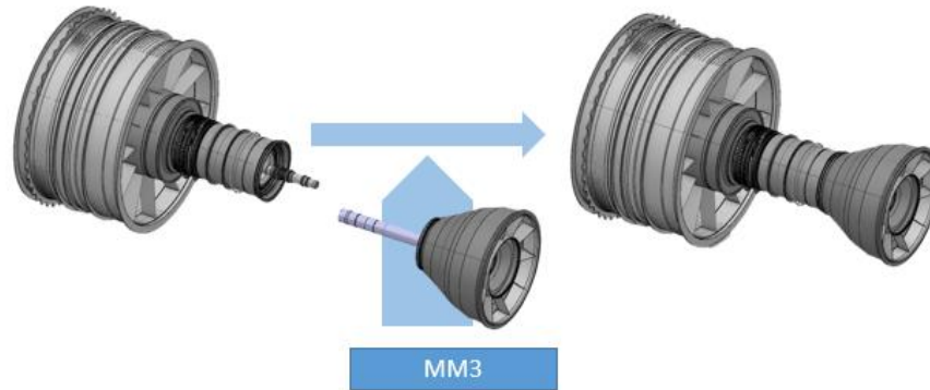
Fig. 7: Brief diagram of the assembly sequence in Station 2.
