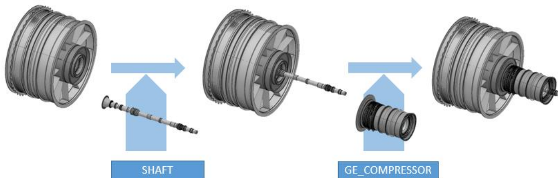
Fig. 6: Brief diagram of the assembly sequence in Station 1.
