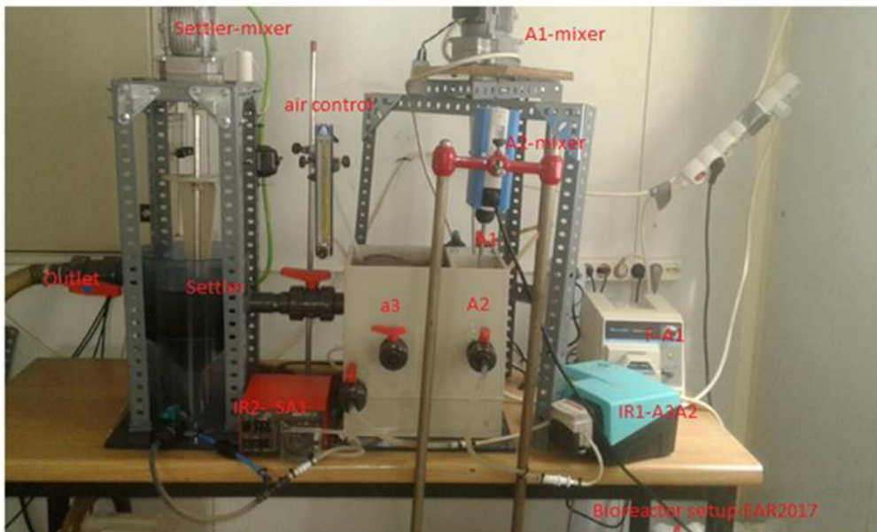
Figure 2. Schematic photo of the integrated bioreactor (A1-anaerobic, A2-anoxic, A3-aerobic and settler)
