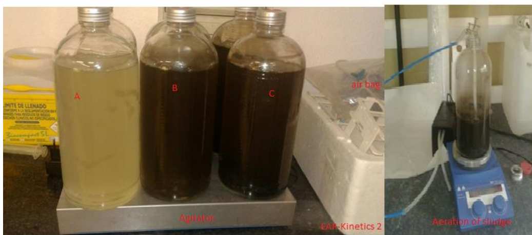
Figure 4. Schematic photo of the experimental setup used for S kinetic oxidation experiments (left picture) and aeration sludge system (right picture)
