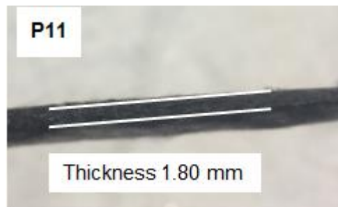
Fig. 3.5: Final thickness with the hand-press at 90°C.
