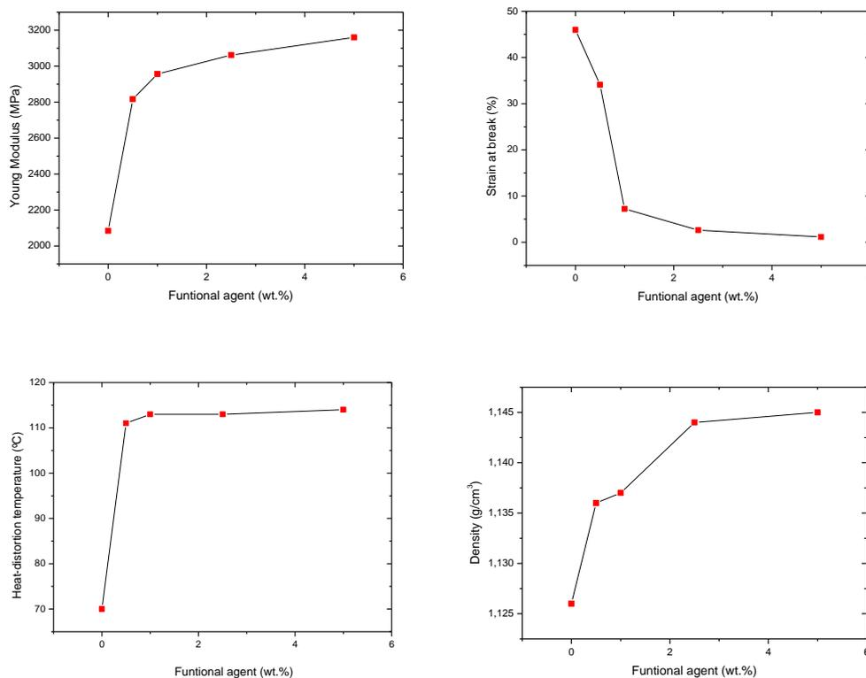
**Figure 3.** a) Young modulus, b) strain at break c) heat-distortion temperature and d) density versus functional agent content
