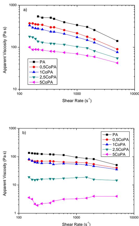
Figure 2. Apparent viscosity of star-shape polyamides by capillary rheometry versus shear rate: a) 230°C and b) 260°C
