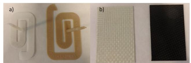
**Figure 4.** a) Injection moulding tests of PA and 5CoPa using pressure-limit control. b) Structural thermoplastic composites based on glass-fibre and carbon fibre by film-stacking process.
