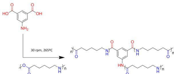
Figure 1. Molecular structure of star-shape polyamide
