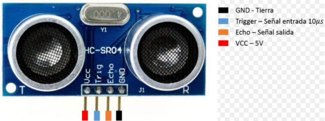
Figure 24 pinout of the HC-SR04 [14]
