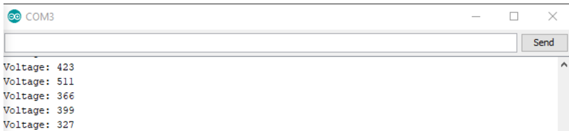
Figure 74 Potentiometer analogRead() with 6 bits of resolution with 5 V
