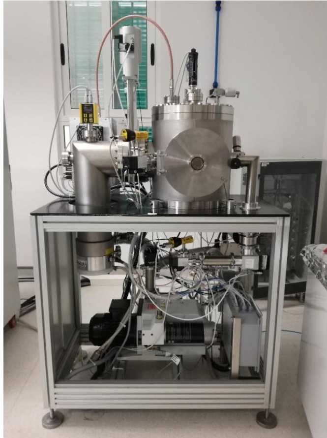
Figure 33. Set up of the PECVD
