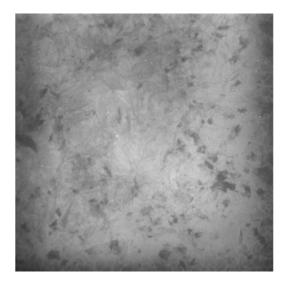
Figure 1. PL image of a mc-Si wafer.
