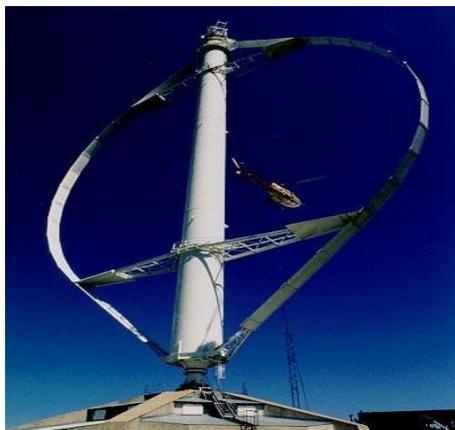
**Figura 1-5 Rotor Darrieus [<http://opex-energy.com>]**
