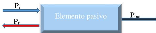
FIGURA 10. ELEMENTO PASIVO CON ONDA REFLEJADA
