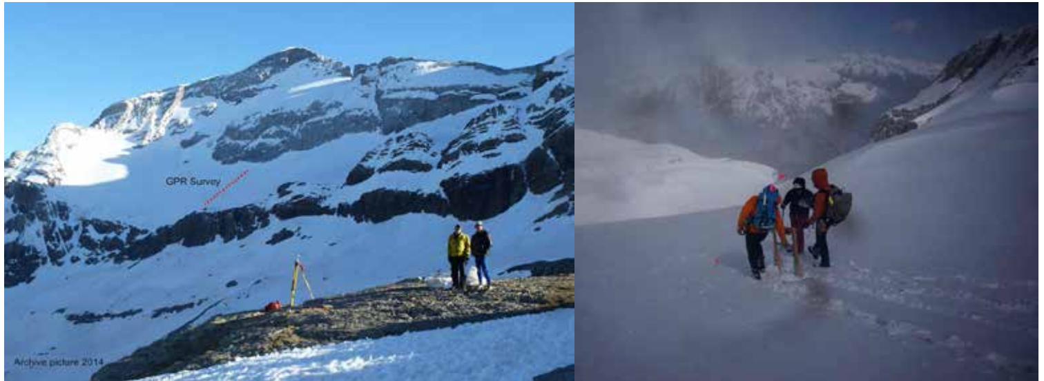
Figure 1.- Photographs of the study area in Monte Perdido Glacier (above) and data acquisition with 200 MHz GPR (below).
