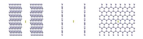
Fig. 1 – Three views of a graphene slit-shaped pore with one hydrogen molecule inside. The two graphene sheets are flat and parallel.
