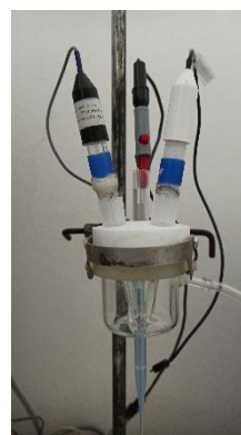
Figure 2. a) \mu AUTOLAB III b) overflow home-made wall-jet electrochemical cell
