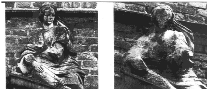
The deterioration of marble due to acid rain is dramatically illustrated by photographs of this statue in Herten, Germany taken in 1908 (left) and 1969 (right).
