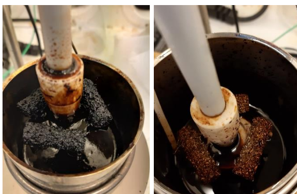
Figure 3.5. Obtained PFA coating: (a) foamy dark polymer obtained when sudden rising of temperature takes place, (b) golden polymer obtained when not sudden rising of the temperature takes place.
