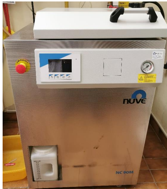
Figure 3-1. Autoclave for moist heat and dry heat sterilization.
