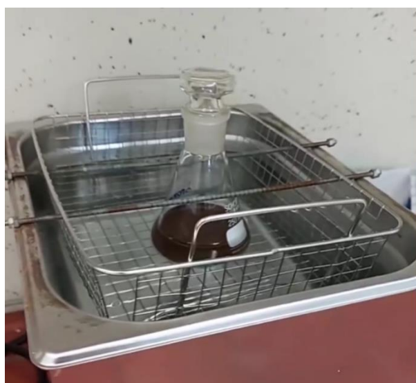
Figure 10.- Set-up for the ultrasound extraction
