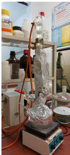
Figure 9.- Set-up for the Soxhlet extraction
