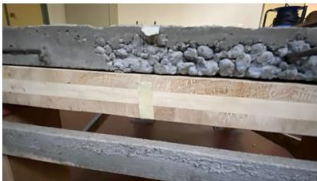
Figure 7 - Slab on wooden structure and placement of accelerometers
