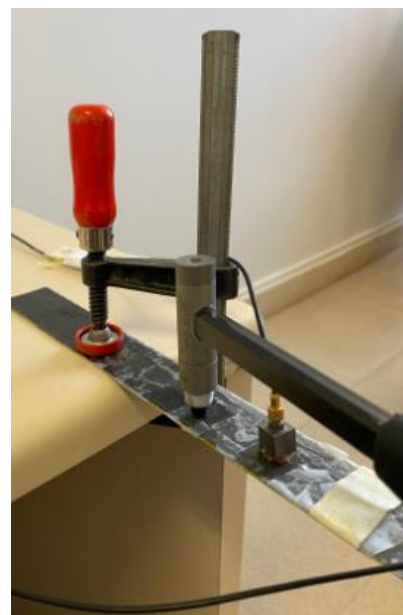
Figure 2 - Modal test by impact hammer
