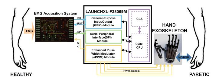
FIGURE 3. Simplified block diagram of the EMG-driven control of RobHand for assisted bilateral therapy.
