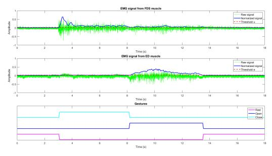
FIGURE 6. EMG signal treatment of the bio-controller for the proposed threshold EMG-driven control: raw EMG signals of ED and FDS muscles, normalized EMG signals, thresholds and determined gestures.
