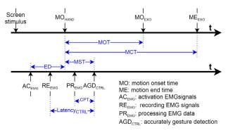
**FIGURE 9.** Timing diagram showing the following time parameters: MST, MOT, MCT, ED, CPT and Latency<sub>CTRL</sub>.
