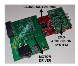
FIGURE 2. LaunchXL-F28069M connected to the motor driver and EMG acquisition system boards.
