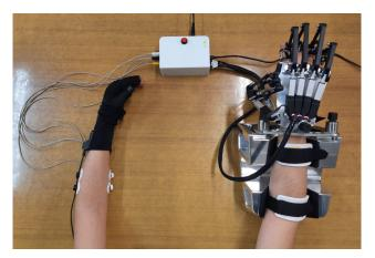
FIGURE 8. Experimental setup. The subject (left-handed) is wearing the 5DT data glove on her dominant hand and the exoskeleton on her non-dominant hand, while recording the EMG signals of the target muscles of the forearm of the dominant hand.
