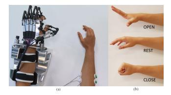
FIGURE 7. Bilateral assisted training with the RobHand exoskeleton, which replicates three predefined hand gestures.
